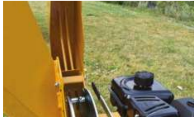
Fixed gate for consistent, fine mulch
