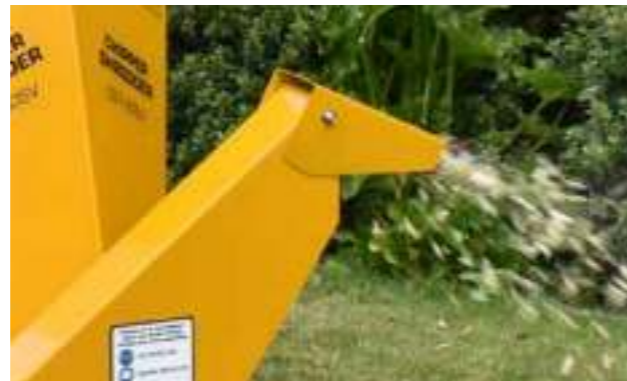
High exit chute for discharging into trailer or onto gardens
